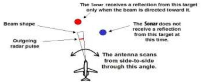
Fig. 4. Finding targets direction
