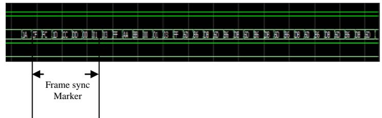
Figure 12. Frame with sync marker
