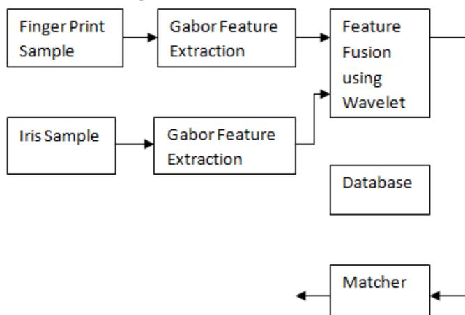
Fig 1 Block diagram of a Multimodal biometric
