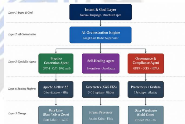
Figure 2. ADPO System Architecture showing the five-layer hierarchy from intent specification (Layer 1) through the AI Orchestration Engine (Layer 2), Specialist Agents (Layer 3), Runtime Platform (Layer 4), and Storage Zone (Layer 5).
