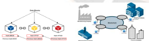
Fig. 2(a) Architecture of Blockchain Technology, 2(b) Blockchain and ERP systems
