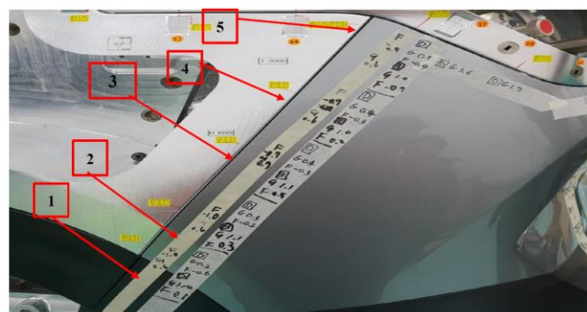
Fig 1: Gap present between the bumper and body on the left-hand side.
