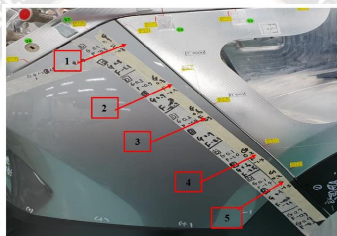
Fig 2: Gap present between the bumper and body on the right-hand side.
