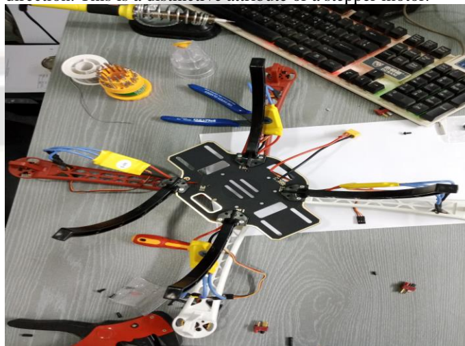
Figure 19 Complete Wiring of the Flight Control Board, Receiver, and the Motors
