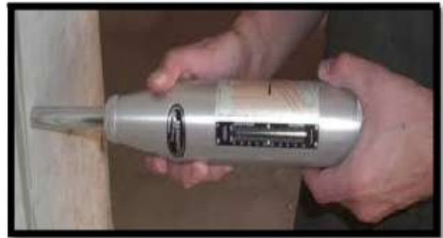
Fig.7 Rebound hammer test
