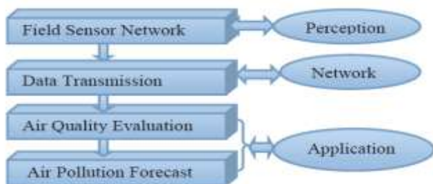
Fig 2: IOT based air pollution monitoring and forecasting system
