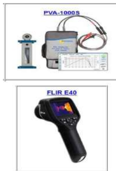
Fig. 2 I-V Curve Tracer and Thermal Imaging Device
