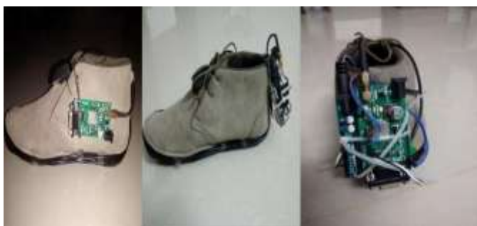
Fig. 6. Wearable GPS Shoe Demonstration
