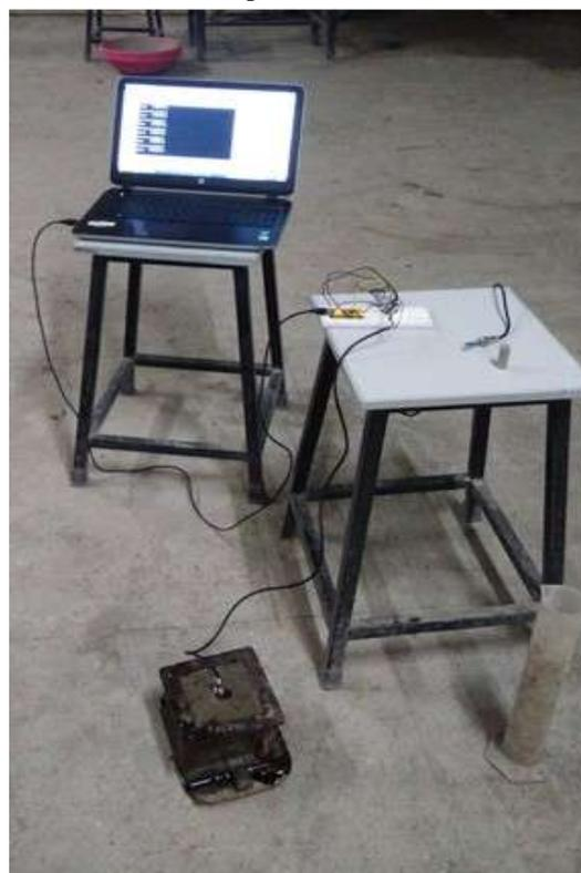
Fig. 4. Sensor mounted in concrete and data acquisition.
