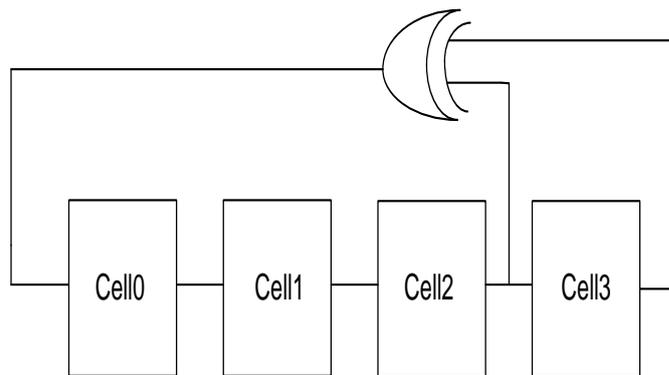
Fig 5 Test Pattern generator
