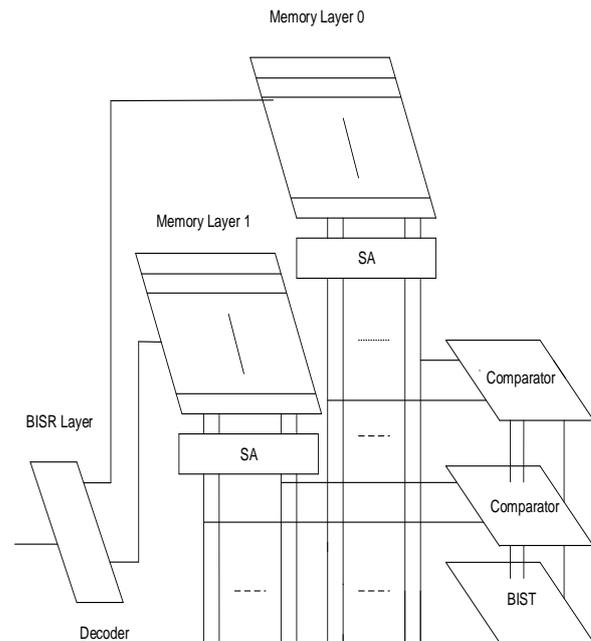
Fig 13. Built-in Self-Repair Architecture for 3D Memories
