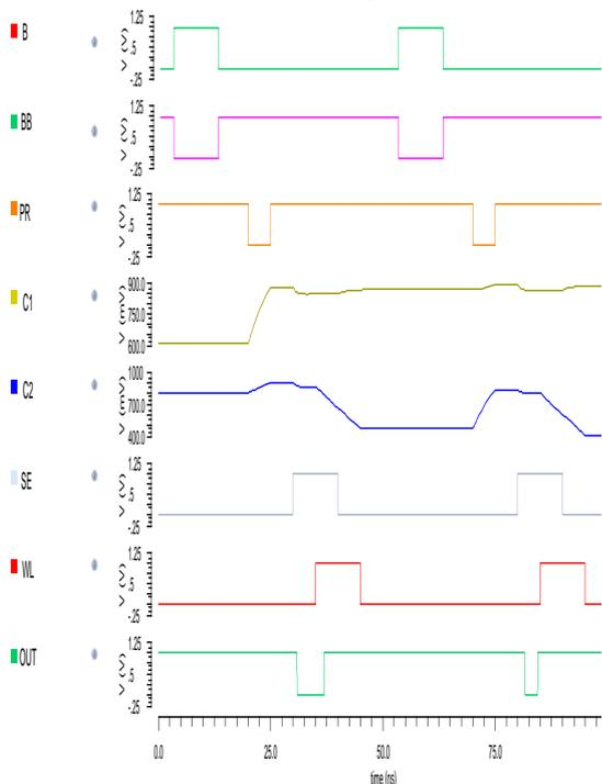
Fig 4. SRAM read operation
