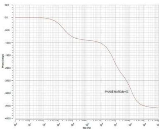
Fig. 7 Measured open-loop frequency response at V<sub>DD</sub>=0.75 V
