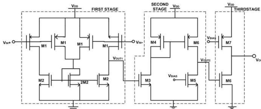
FIG. 4. Three-Stage OTA with separate biasing and without frequency compensation
