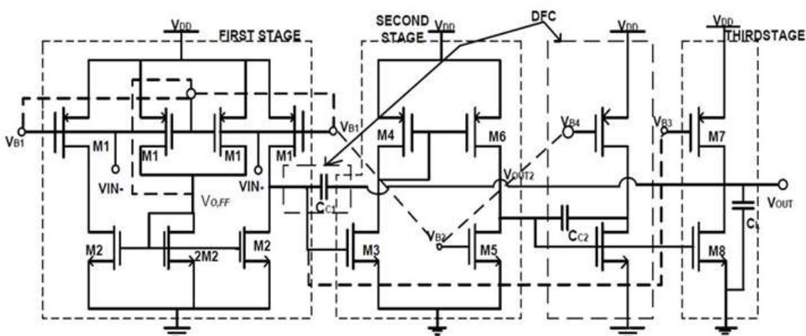
FIG. 5 OTA with self-biasing and frequency compensation
