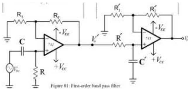
Figure 01: First-order band pass filter
