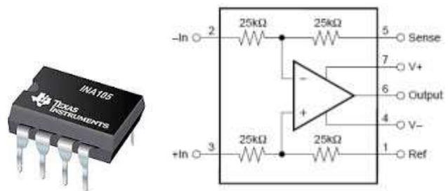
Figure 1.2: INA 105 PINOUT
