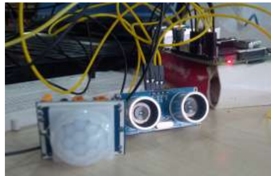
Fig: working diagram of Ultrasonic + PIR sensor.
