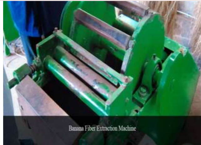
Fig no.3 shown horizontal blades weld on roller
