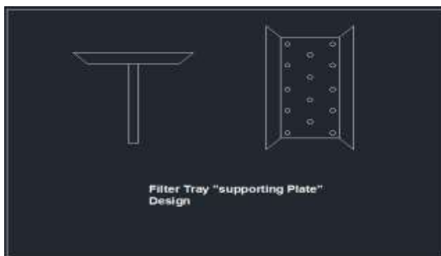
Fig No.6 Filter Tray Supporting Plate Design
