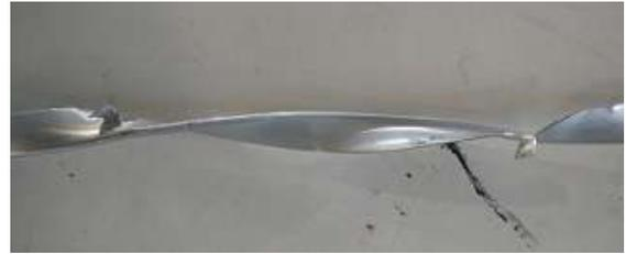
Figure 3. Jagged Twisted Insert
