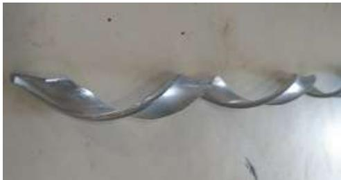
Figure 1. Simple Twisted Insert
