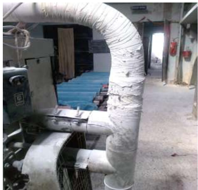
Fig.9 - Photograph of Change in Suction Port Position
