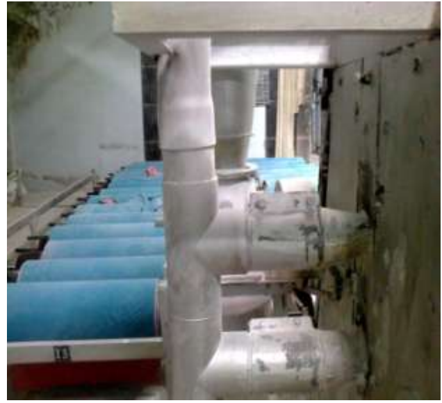
Fig.7 - Photograph of Change in Suction Port Position
