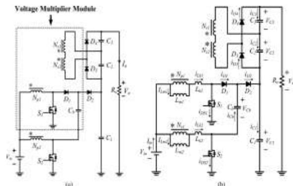
Fig.3(a) Converter with voltage multiplier module. Fig.3(b) Proposed Converter
