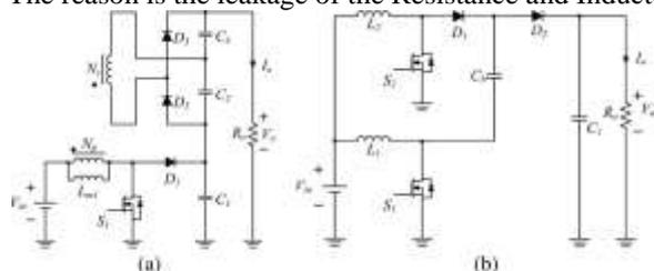
Fig.2 Modified Boost flyback Converter
