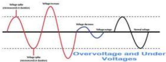
Fig.6 Under voltages and over voltage
