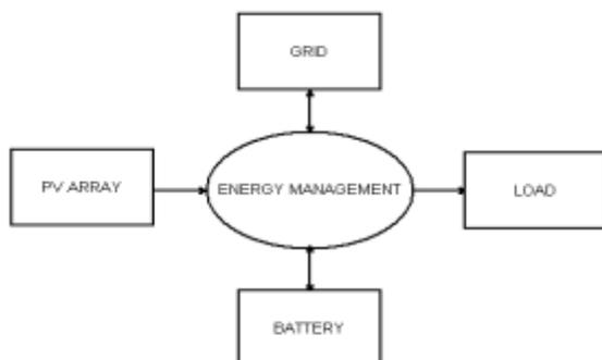
Figure. 1 Block diagram of multi energy system with energy management
