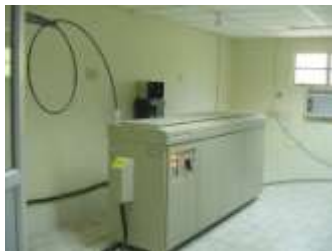
Figure 1. Solid state Nd:YAG Laser source at WRI used for experimental work [18].
