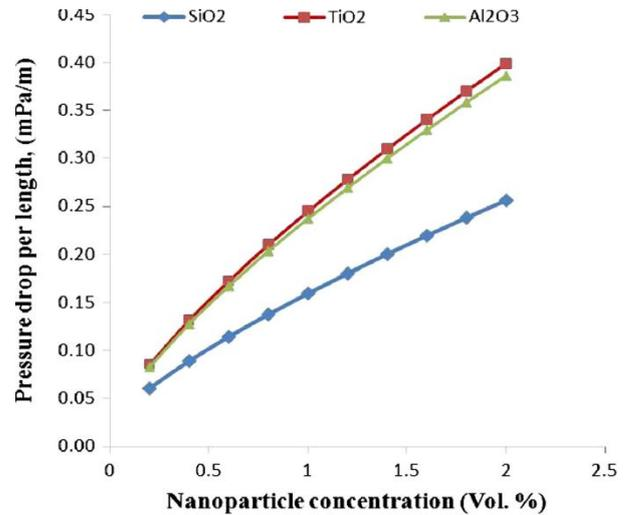
Fig 3..Pressure drop per unit length for different nanofluids[10]
