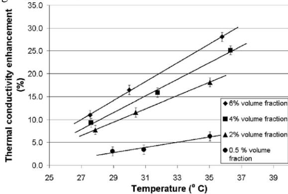
Fig 5. Temperature vs thermal conductivity at different volume fraction[12]
