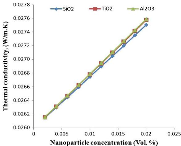
Fig 2. . The thermal conductivity at different volume fraction[10]
