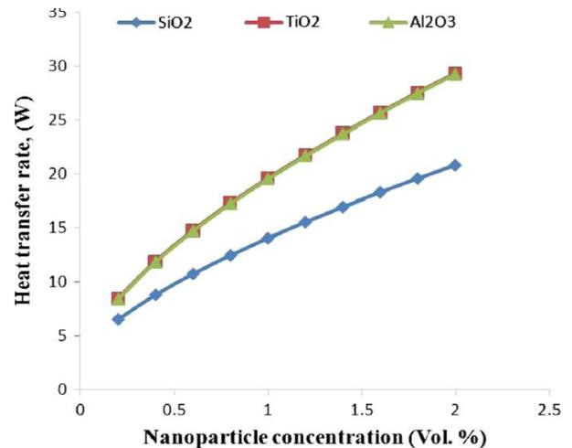
Fig 4. Heat transfer rate of plate fin heat exchanger with different nanofluids[10]
