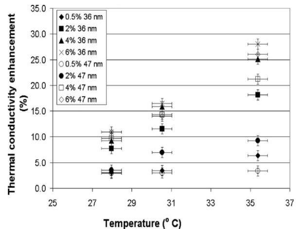
Fig 6. Temperature vs thermal conductivity at different volume fraction of 36nm and 47nm nano size particle.[12]
