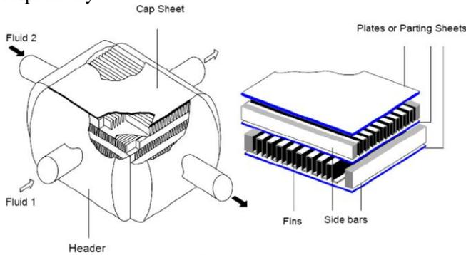
Fig.1 Plate fin heat exchanger[10]
