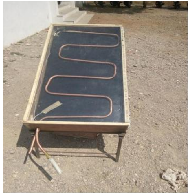
Fig 1. Fabricated set up of Double pass solar air heater
