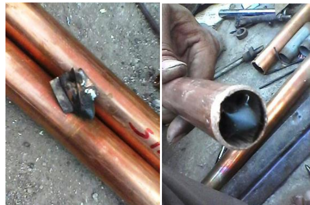
Fig.4 Nozzle shape arrangement at entrance of pipe.
