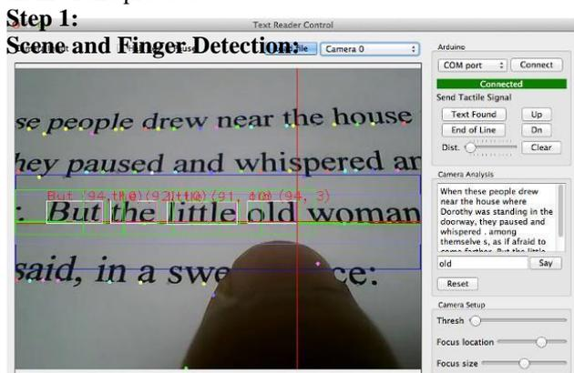
Figure 4: Our software in midst of reading, showing the detected line, words and the accumulated extracted text.
