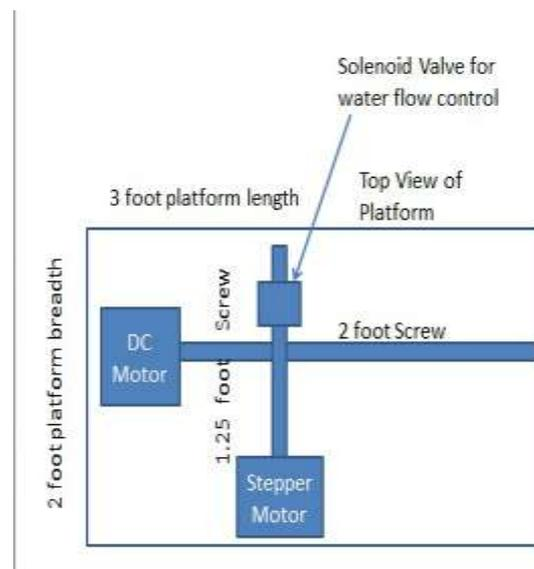
Fig. 2: Top view of the prototype
