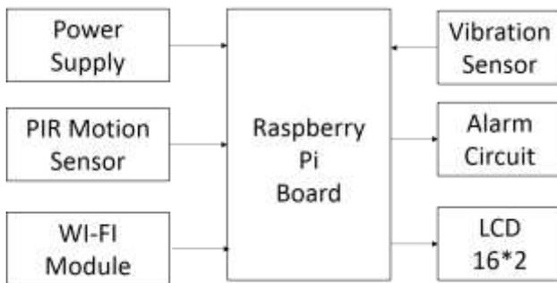
Proposed system includes RPi board with PIR sensor, vibration Sensor for sensing in security system and the notification will be available on the email or owner and Push eta application in smartphones with buzzer in present system.
