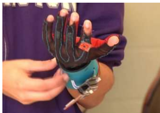
Figure(1):Sensors on the outside of the glove data of which is sent to the database
