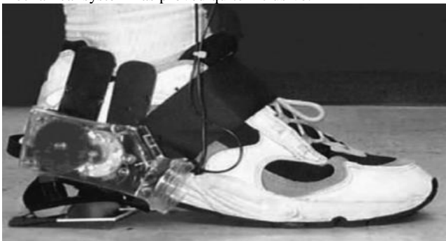
Figure 7. Rotating generator adapted in a shoe [18]
