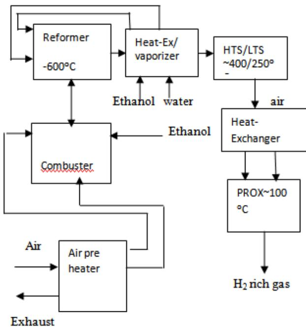
Fig1:- Diagram for integrated reactor for steam reforming of Ethanol
