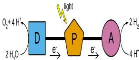
Fig4:- Triad assembly that produce Hydrogen using photosynthesizer
