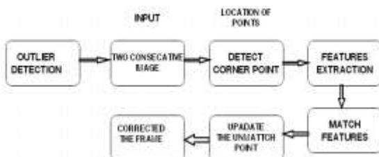
Figure 2.9 Steps for outlier’s detection and remove
