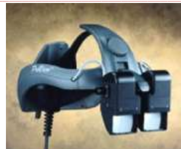
Figure 2: Optical See-Through HMD.
