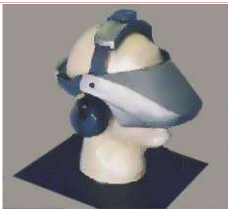
Figure 7: Video See-Through HMD.
