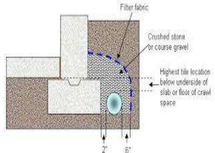
According to this methodology subsurface drain system is prepared.[7]
