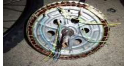
Inside view of BLDC hub dc motor.
