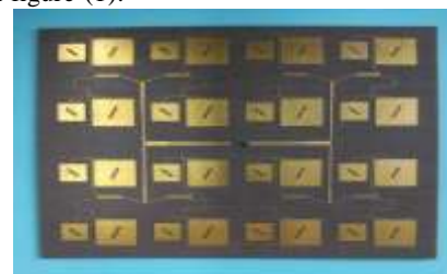
Fig. 1 Structure of the dual-band dual-CP array with conventional feed network: fabricated 4x4 element array.
