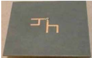
Fig.7. Final antenna layout fabricated on RT/Duroid 5880
