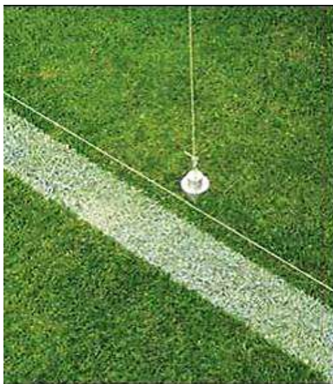
Fig 6 Final installation test – dropping a plumb to define the goal line.
