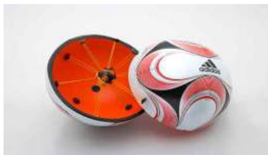
Fig 1 The Adidas Teamgeist – II with implanted chip, part of proposed Cairo-Adidas system for Goal-line technology
