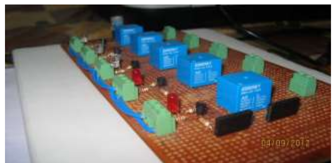
Fig .5 Relay board
