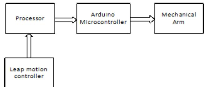
Fig. 1 Block Diagram of hand gesture controlled robotic arm
