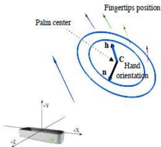
Fig. 6 Data acquired by the Leap motion
