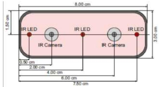
Fig. 3 Schematic view of Leap motion controller
