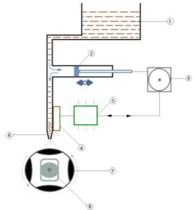
Fig. 2. Lubricant Injector
