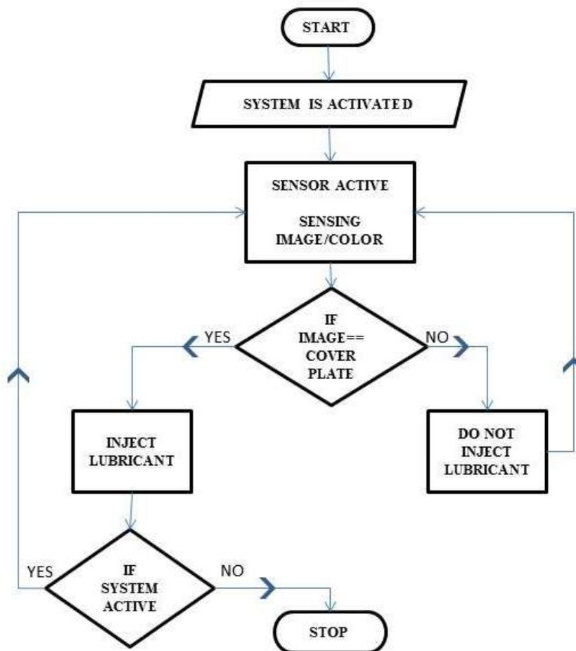
Fig. 3. PLC working Flowchart
