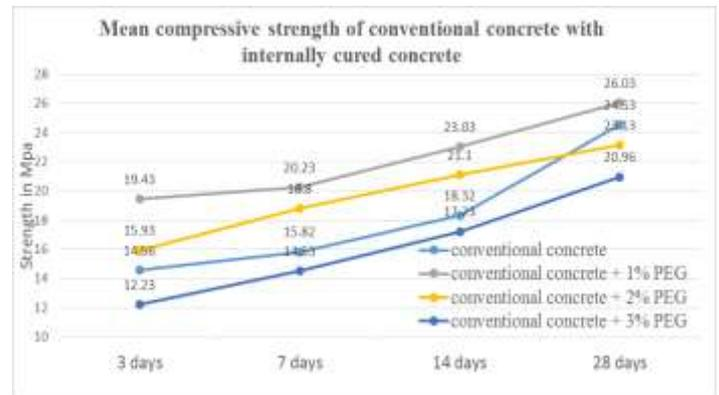
Fig 1: compressive strength for internally cured and conventional mixes
