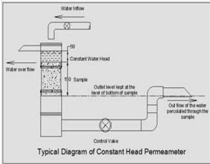
Fig. 1: Typical diagram of Constant head Permeameter used to determine permeability of pervious concrete specimens
