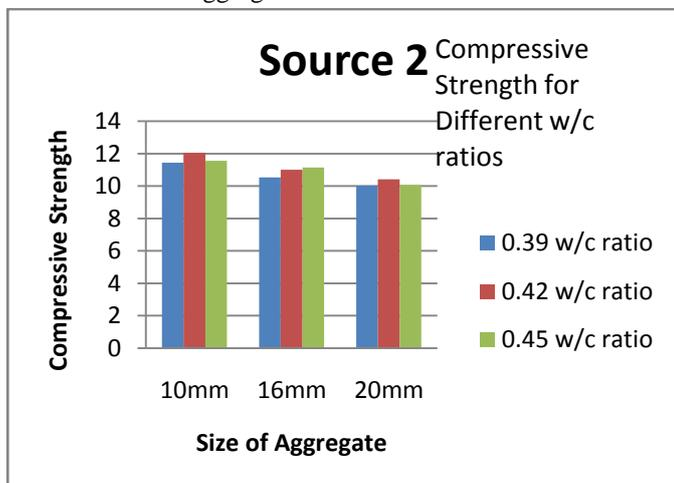
Fig.3 Compressive Strength For Different Size Of Aggregates And W/C Ratio
