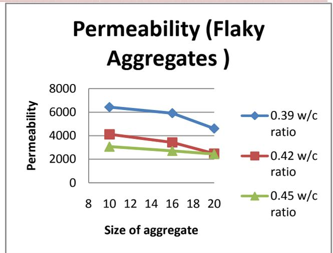
Fig.4 Permeability for Different Size of Aggregate And Different W/C Ratios
