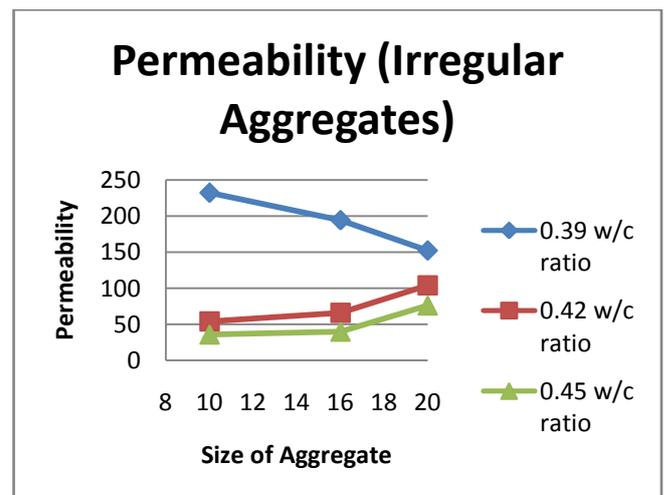
Fig.6 Permeability for Different Size of Aggregate And Different W/C Ratios
