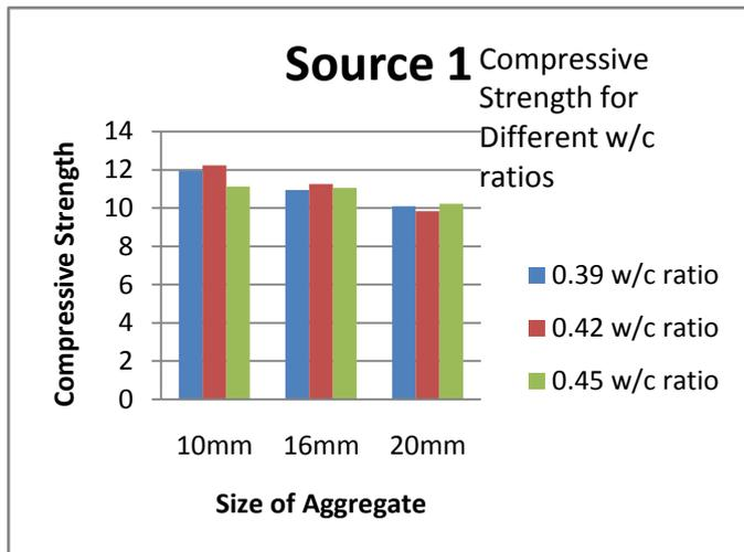
Fig.2 Compressive Strength For Different Size Of Aggregates And W/C Ratio
