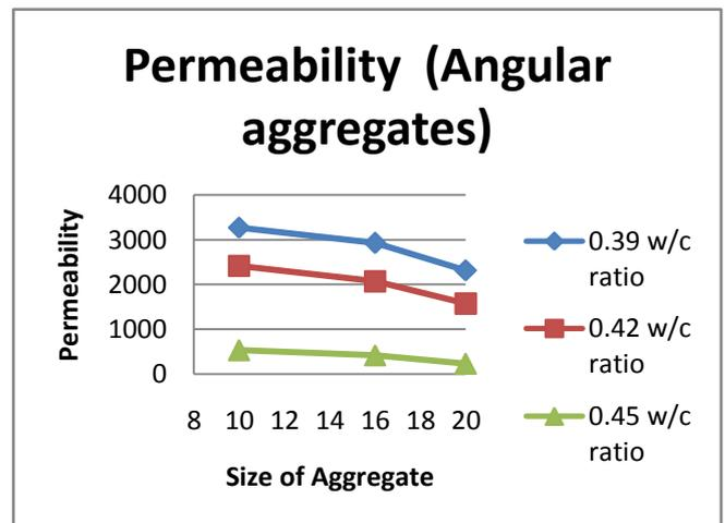
Fig.5 Permeability for Different Size of Aggregate And Different W/C Ratios
