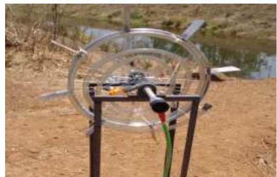
Fig 2. Set up of spiral tube water wheel pump.
