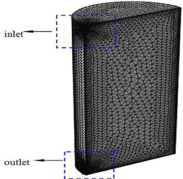
**Fig.2** Computational domain with unstructured grid of the modelled thermal storage tank
