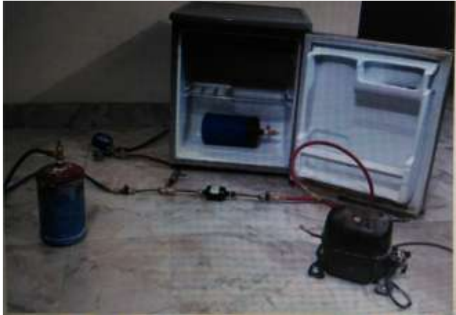
Figure 3: Zeolite-Water Refrigeration Apparatus setup
