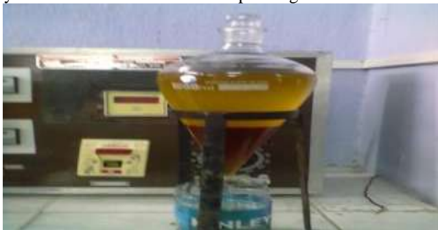
Fig. 2 Settling of base treatment
