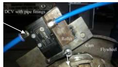
Fig. 3 Photographic view of DCV roller and cam mounted on flywheel
