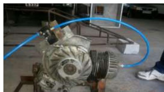
Fig. 4 Photographic view of complete assembly of modified air engine
