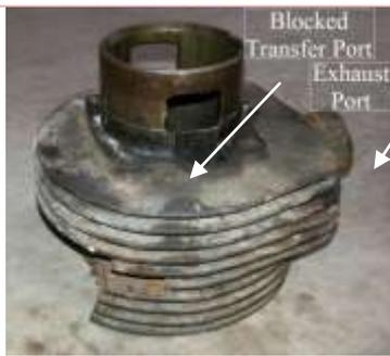
Fig. 1 Photographic view of Cylinder block after modifications
