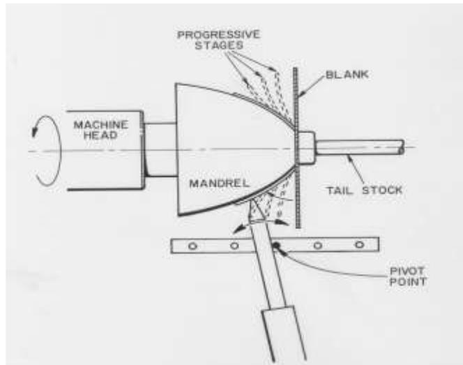
Figure 1 Conventional Manual Spinning [1].
