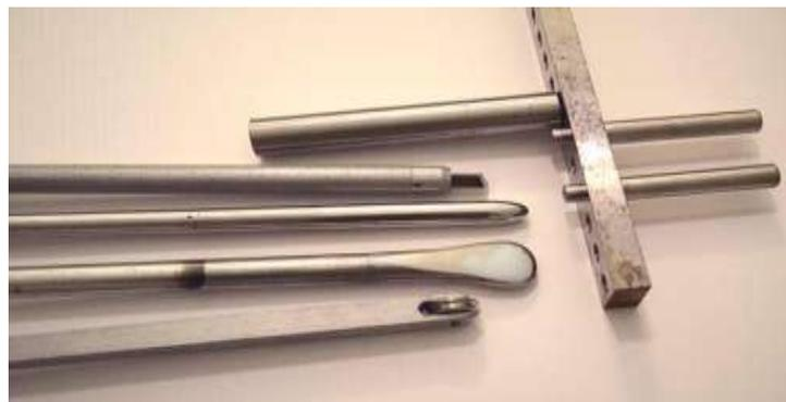
**Figure 12 Tools and Tool post for Metal Spinning**
