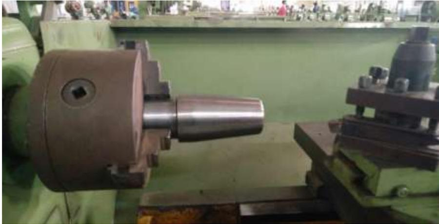
Figure 6 Mandrel in Setup
