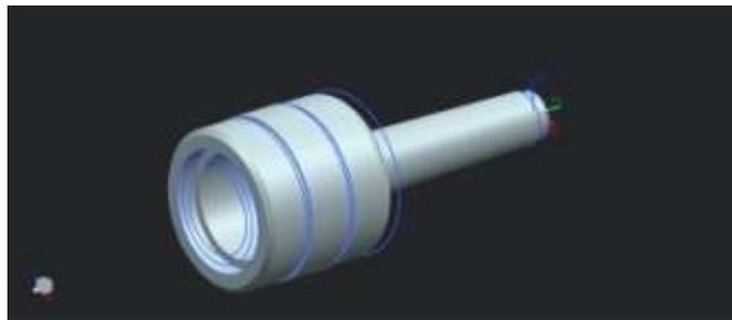
Figure 7 CAD view of Live Centre Bore
