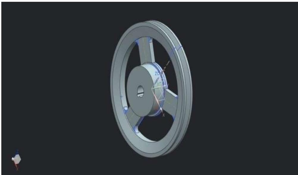
Figure 9 CAD view of Pulley
