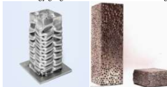
Fig. IV steel crash box [7] Fig. V structure of metal foam crash box [7]
